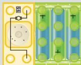
**3. Motor (95):** Place the motor across the battery holder (95 at top) as shown; it should spin clockwise.
