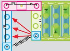
Wire Block tests - Insert the Wire Blocks between the spring wire to lamp connection shown in the figure. The lamp should light.
