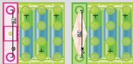
**2. Wire Blocks (1-5), Spring Wire (9), and Speaker (95):** Use this mini-circuit to test each of the Wire Blocks and Speaker (95), one at a time. The lamp (76) should light if the part is functioning properly. Follow the steps below:
